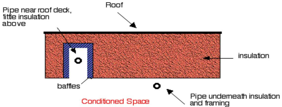
CPVC pipe and spray foam are chemically compatible. There have been concerns regarding whether the spray foams' exothermic heat would soften the glue joints. While there is no evidence of this being a problem when the foam is properly applied, wrapping the pipe joints with fiberglass before applying spray foam should be done as a precaution and is generally installed by the insulation contractor.
